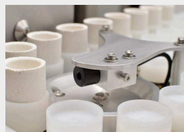
Autoloader with acid-resistant plastic crucible holders
